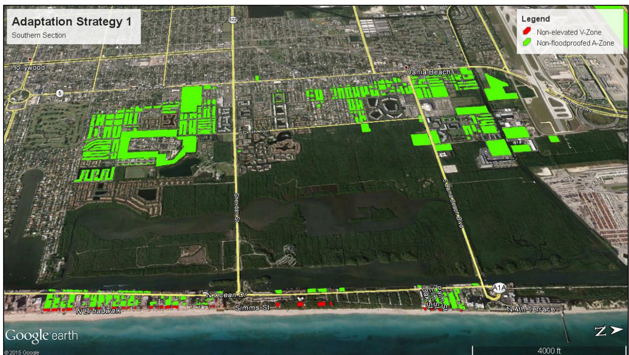
Fig. 21. Non-elevated buildings in FEMA V-Zone (red) and non-floodproofed buildings in FEMA A-Zone (green) – southern section of study area.
