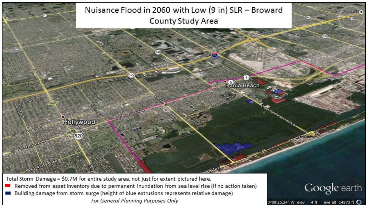
Fig. 10. One-time damage estimate for nuisance flood in 2060 with low sea level rise.
