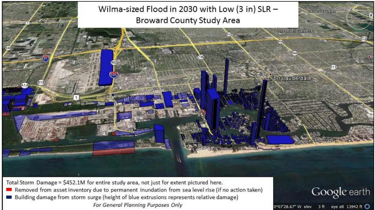
Fig. 13. One-time damage estimate for Hurricane Wilma-size flood in 2030 with high sea level rise.
