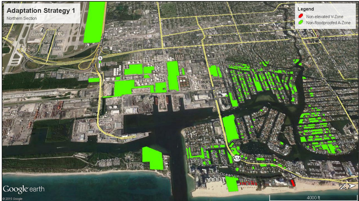
Fig. 21. Non-elevated buildings in FEMA V-Zone (red) and non-floodproofed buildings in FEMA A-Zone (green) – southern section of study area.
