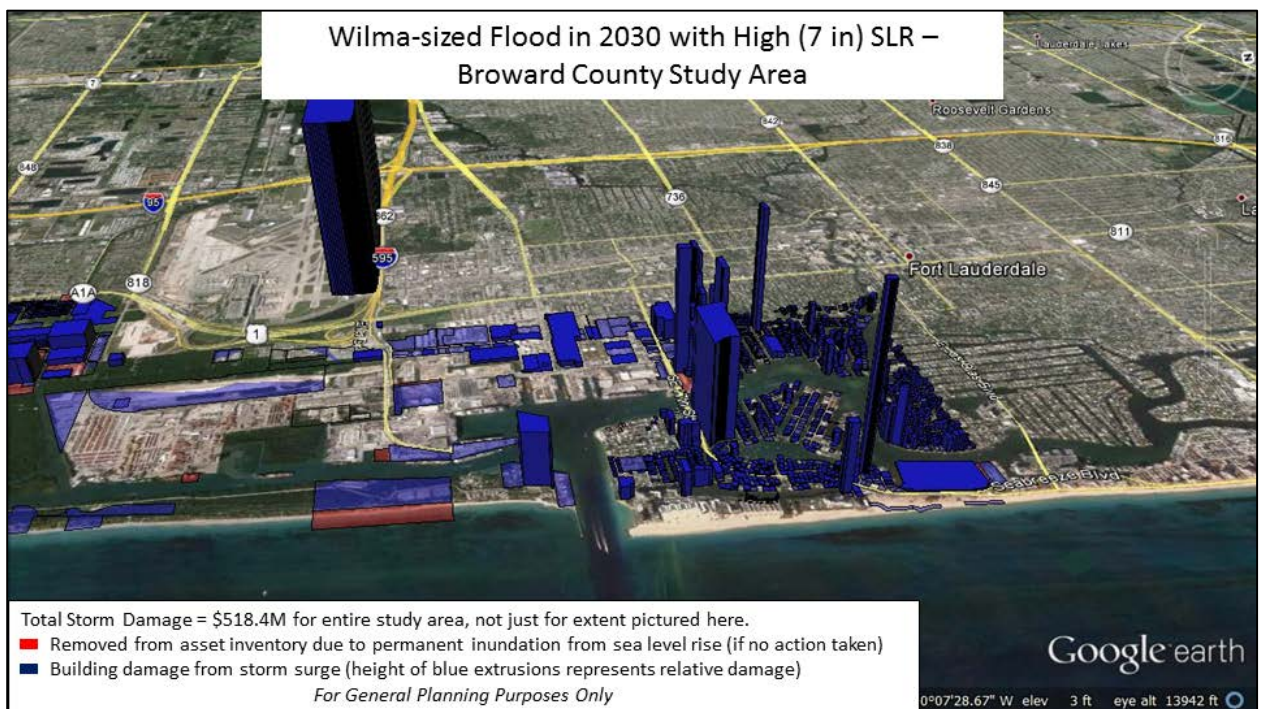
Fig. 13. One-time damage estimate for Hurricane Wilma-size flood in 2030 with high sea level rise.
