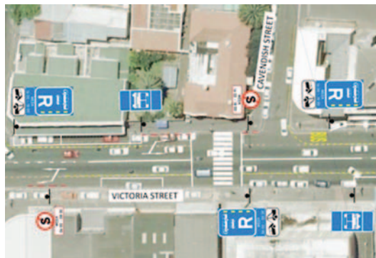
This drawing demonstrates how dedicated curbside bus lanes can be conditioned to separate bus service from other traffic. Similar treatments were used for the bus and minicab priority lanes along Victoria Street in Cape Town.
