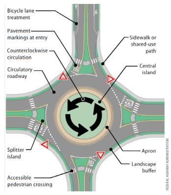
A roundabout is a type of circular intersection. Roundabouts have been proven safer and more efficient than other types of circular intersections.
