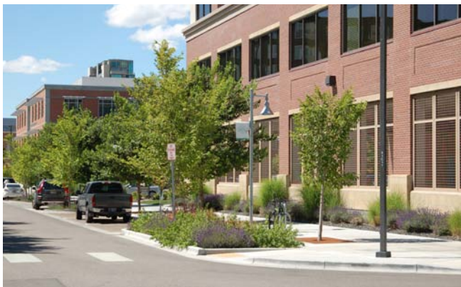
Broad Street in Boise, Idaho's Central Addition LIV District incorporates stormwater infrastructure (such as permeable pavers, rain gardens, and swales) in the public right-of-way to help the surrounding properties meet their stormwater management requirements.
